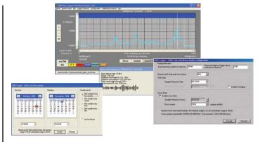
Logger programming is easily achieved by using the 'Setup' dialog, which allows the user to choose Start and End times, Sampling Rate, Averaging, Thresholding, as well as synchronize the logger with the PC clock. The setup dialog also indicates the expected battery and memory usage for the chosen deployment settings.
