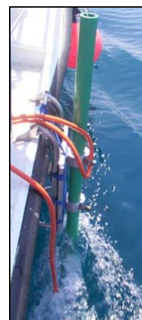
SES-96 light operated on a rubber boat. On the right hand picture the metal plate supporting the pipe can be seen, this time fixed at a ladder on board of a small motor yacht. (Photos courtesy of FSU Jena)
