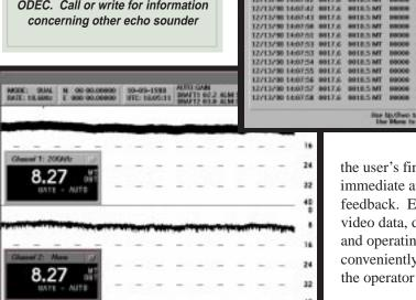
All collected hydrographic survey data are position and time tagged. A heave-compensated chart record is presented to the user. A standard, internal, non-volatile data logger memory is capable of storing up to 2.5 hours of analog water column and 8 hours of digitized depth data for playback on the LCD display, or printing to an external device.
